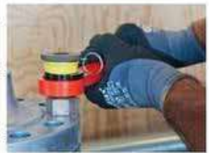
Reposition wrench on nut and release spring loaded plate and continue.
