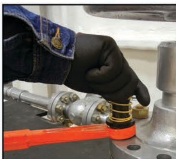
Screw the HAMMERTIGHT wrench retainer onto the stud. At least two threads of the stud must be engaged into the retainer.
