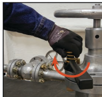
Screw HAMMERTIGHT wrench retainer onto the stud, again making sure at least two threads of the stud are engaged into the retainer.
