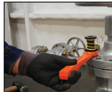
Leaving the HAMMERTIGHT wrench retainer engaged on the stud, lift up on the wrench to reposition.
