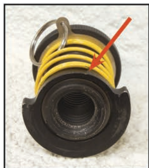
When using offset striking wrenches, place the notch of the retaining plate facing the wrench handle as shown.
