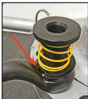
When using offset striking wrenches, place the notch of the retaining plate facing the wrench handle as shown.
