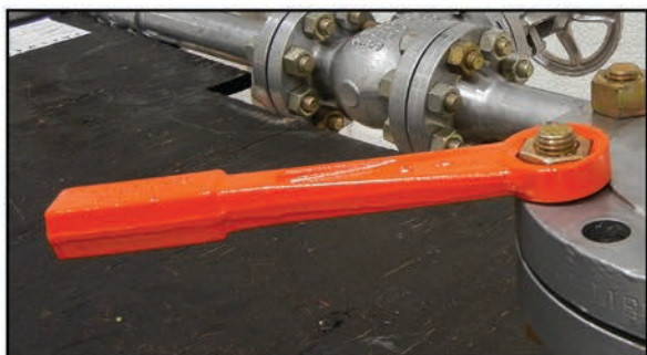
Place wrench all the way down on nut.
