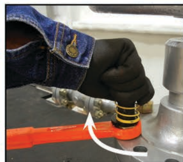
Screw the HAMMERTIGHT wrench retainer onto the stud. At least two threads of the stud must be engaged into the retainer.
