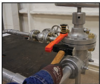
Place wrench all the way down on nut.
