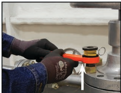
Leaving the HAMMERTIGHT wrench retainer engaged on the stud, lift up on the wrench to reposition.
